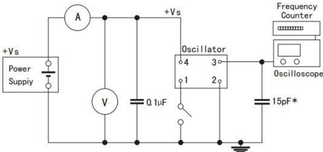
Tri-state: PIN 1 connected to Vdd or floating, the product is working properly; connected to
